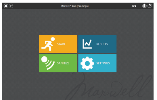
Figure 55. Maxwell® CSC ‘Home’ screen. Selecting Results opens the Maxwell® CSC ‘Results’ screen from which extraction reports from all extraction runs, service activities and system activities can be viewed.
