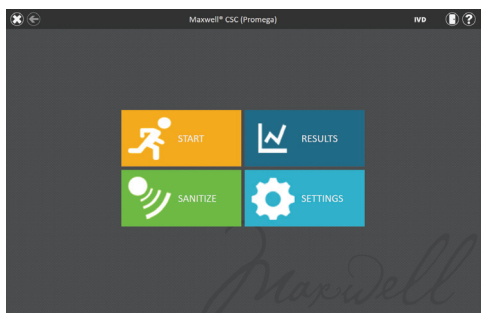
Figure 58. ‘Home’ screen. Selecting the Sanitize button begins the process of performing a UV light treatment of the Maxwell® CSC Instrument.
