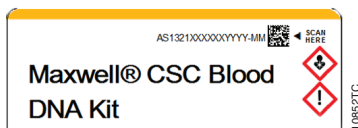
Figure 37. Kit label indicating bar code to scan. Scan the bar code, shown in the upper right of the kit label, to start a purification run.
