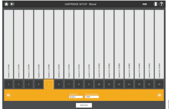
Figure 39. Bar code and kit lot input. By selecting the numbered box at the bottom of any cartridge position, sample ID and kit lot information can be scanned or manually entered for that position. Touching the arrow on the right side of the entry area will move to the next available cartridge position. Selecting multiple positions can be used to enter kit lot information for multiple cartridge positions.
